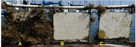
\* A = No Clean Panel; B = Standard Cleaning Panel; C = Manufacturer's Recommended Cleaning Panel
